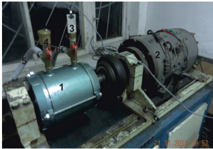
Fig. 3 – Bench for testing: 1 – PMECH; 2 – d.c. motor; 3 – temperature sensor; 4 – deaerator; 5 – tour circuit; 6 – retour circuit.
